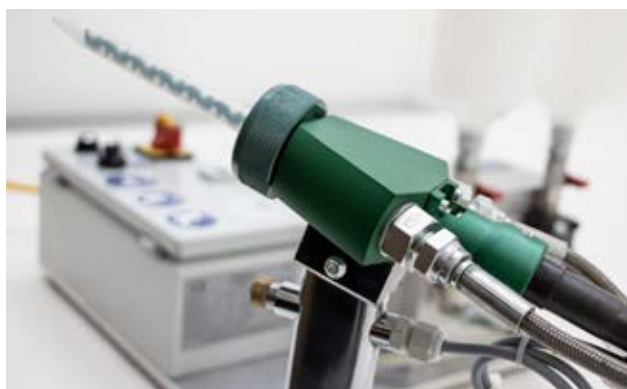
Dynamic mixing with rotating disposable plastic mixer.
